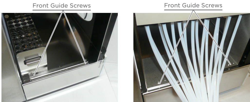
Figure 47 Funnel Rack Installation
