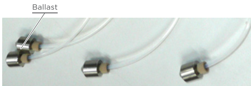
Figure 24 Inlet Tubing Ballasts
