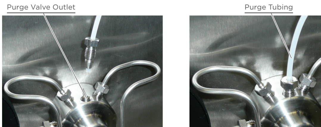
Figure 29 Purge Valve Outlet
